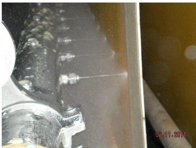
Figure i. High pressure needle showers can effectively cleaning localized sections of the press fabric
