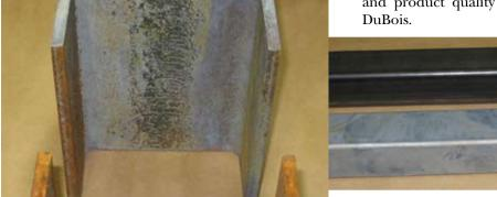
Available in several formulations aimed at various kinds of soils, DuJel cleaners are thixotropic compounds that adhere to surfaces to provide enhanced cleaning of a variety of soil types. Shown here are cleaning results on red rust (left) and mill scale.
