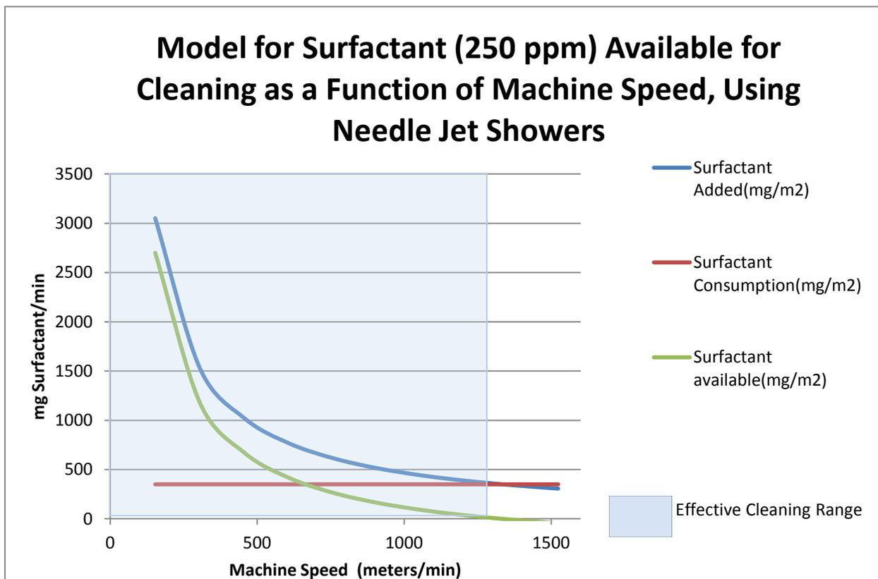
As machine speed increases, more and more of the area of the felt is exposed to the felt conditioner and the effective remaining agent available for cleaning is decreased to the point that at 1300 m/min the surfactant is largely adsorbed onto the press felt and not available for soil emulsification and dispersion. This model will vary by other factors, which include temperature, ionic strength of the water in the
