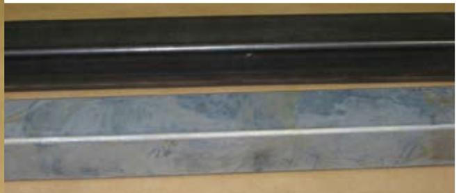
Available in several formulations aimed at various kinds of soils, DuJel cleaners are thixotropic compounds that adhere to surfaces to provide enhanced cleaning of a variety of soil types. Shown here are cleaning results on red rust (left) and mill scale.
