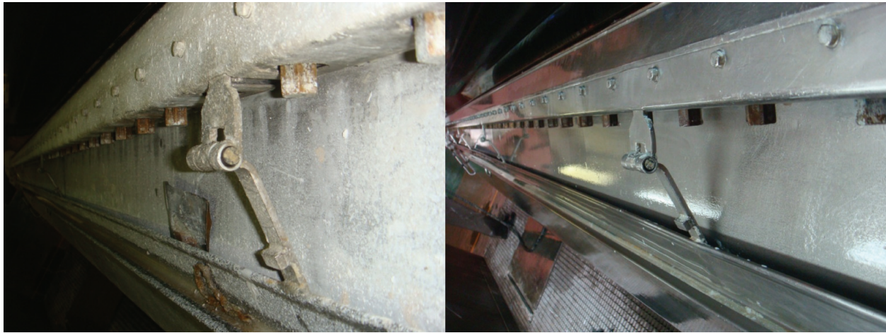
Figure 1. Before (left) and After (right) Photos of Coater Head when cleaned with Stabilized Peroxide Cleaner Product
