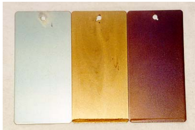
Figure 1: Steel Q-Panels showing range of possible colors produced by iron phosphate
