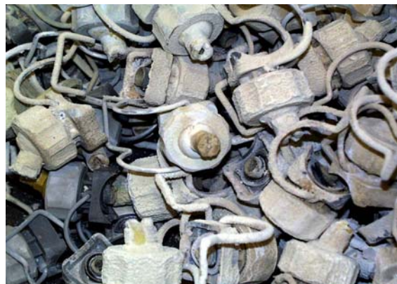
Figure 13: Discarded spray nozzles clogged with insoluble iron phosphate sludge and hard water scale
