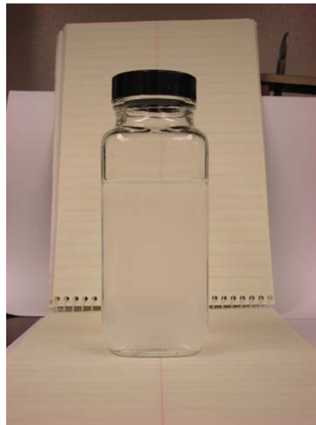
Figure 8: When the pH is above the recommended level, shown here at pH = 6.5, the solution will become turbid indicating active ingredient precipitation
