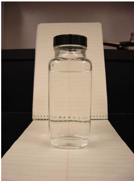
Figure 7: When the pH of a bath is at the proper pH, shown here at pH = 4.5, the solution will be clear
