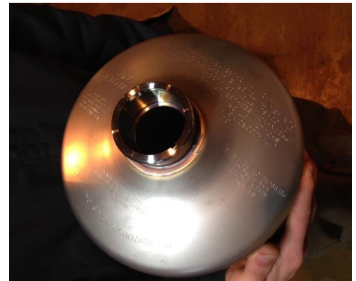
Clean Keg Top Ready for Welding
