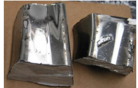
Aluminum wheel pieces before coating removal.
